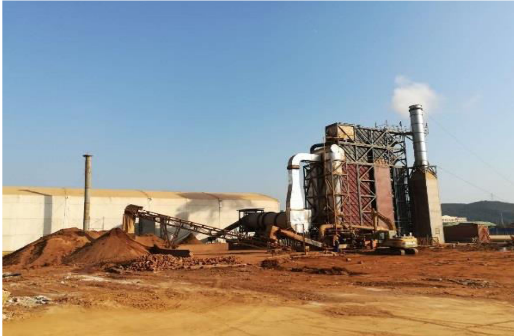
Figure 7: Thermal desorption and high temperature destruction unit at soil treatment site
