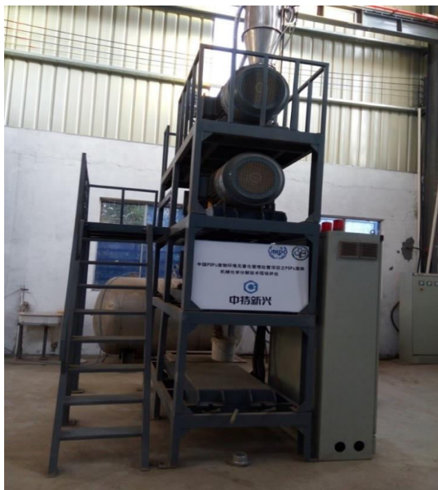
Figure 14: WSM Mechanochemical POPs Polluted Soil Decomposer
